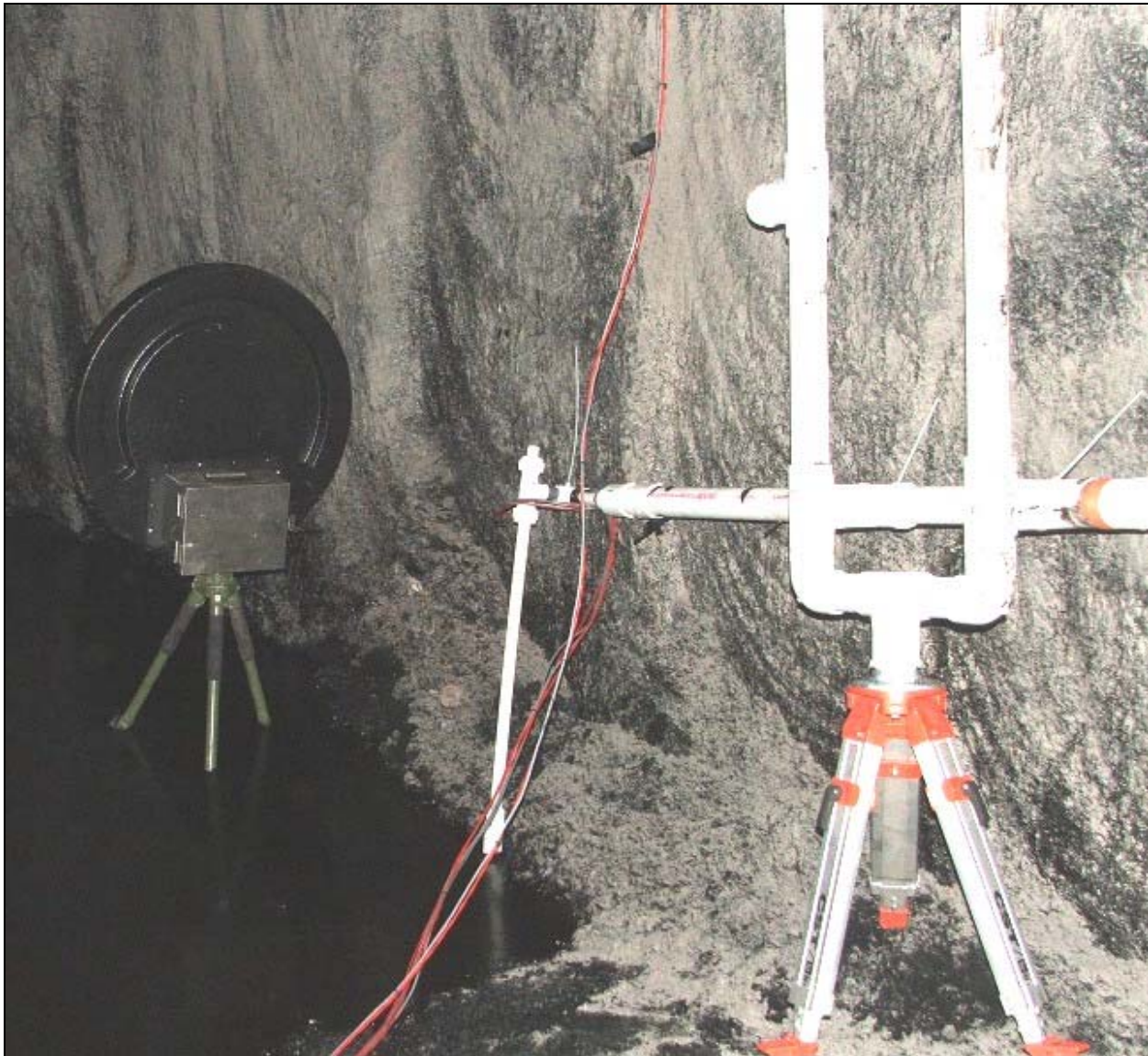
Figure 3-3. The higher frequency induction tool that included a 1-MHz transmitter and a loop antenna receiver was tested in a coal seam.
