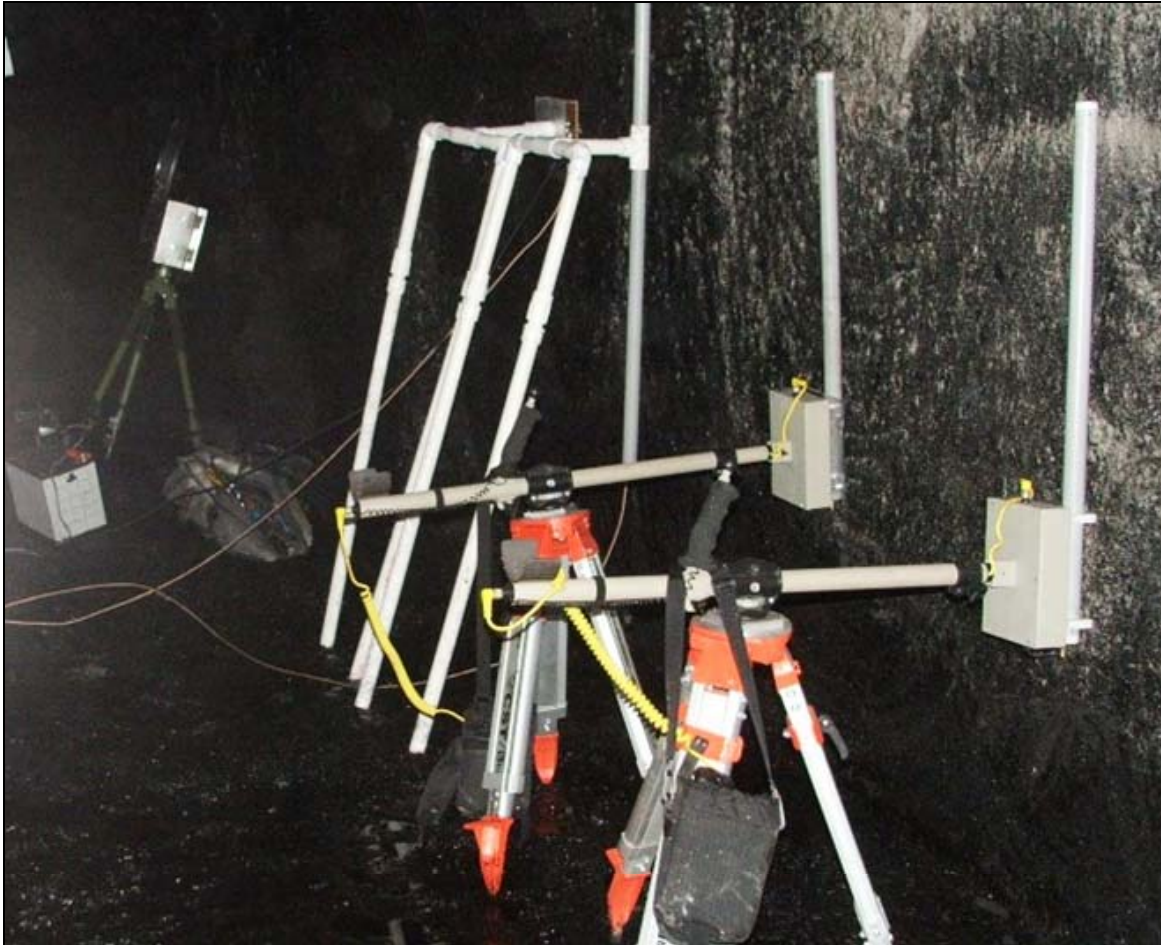
Figure 3-2. Low-frequency, wide-band dipole antennas were also tested with the LAR electronics as independent transmitters and receivers.
