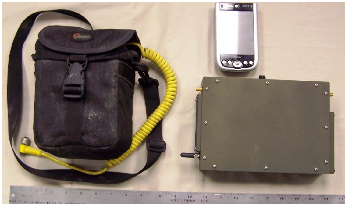
Figure 2-7. SDT electronics, PDA display, and battery pack.
