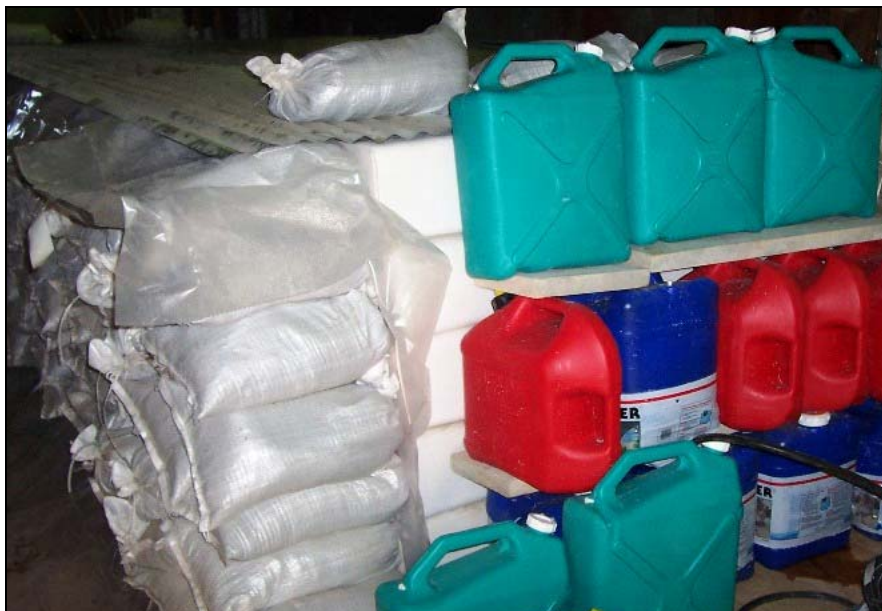
Figure 2-9. Coal seam simulator at the Stolar facility (salt block and sand bag construction). Water jugs provide reflection surface.
