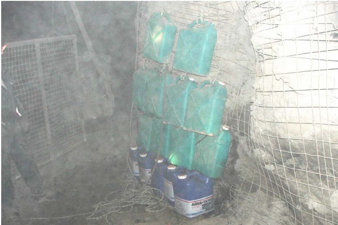
Figure 4-10. A water-coal interface was created on the rib using plastic containers filled with moderately-saline water. The containers created a small reflecting wall opposite of the LAR system at the 20-ft thickness station through the pillar.
