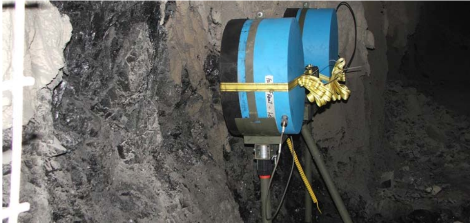
Figure 4-8. LAR prototype system in place against rib at Bowie Static Test Site, February 21, 2007. The transceiver array was placed at several locations moving inby down the rib for data collection through increasingly thick coal seam (on tapered pillar).
