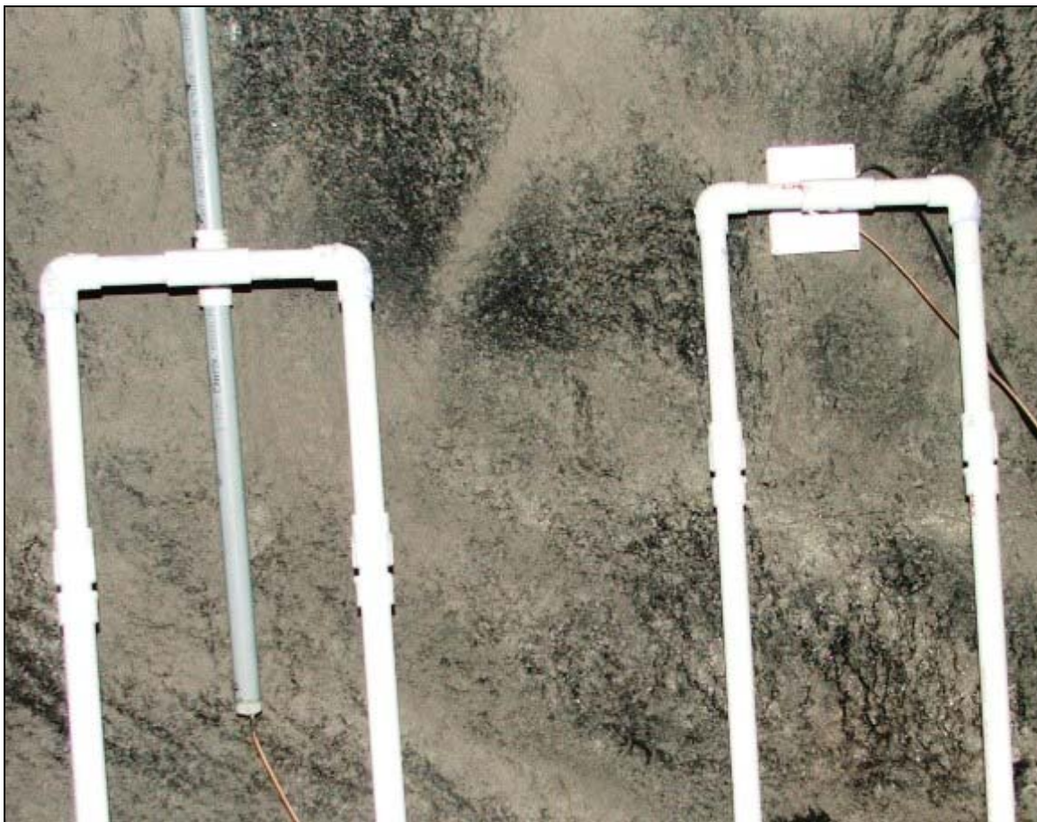
Figure 3-1. Wide-band dipole antennas (left) and RMPA antennas (right) were tested at the Deer Creek Mine. Neither antenna performed to LAR specifications.
