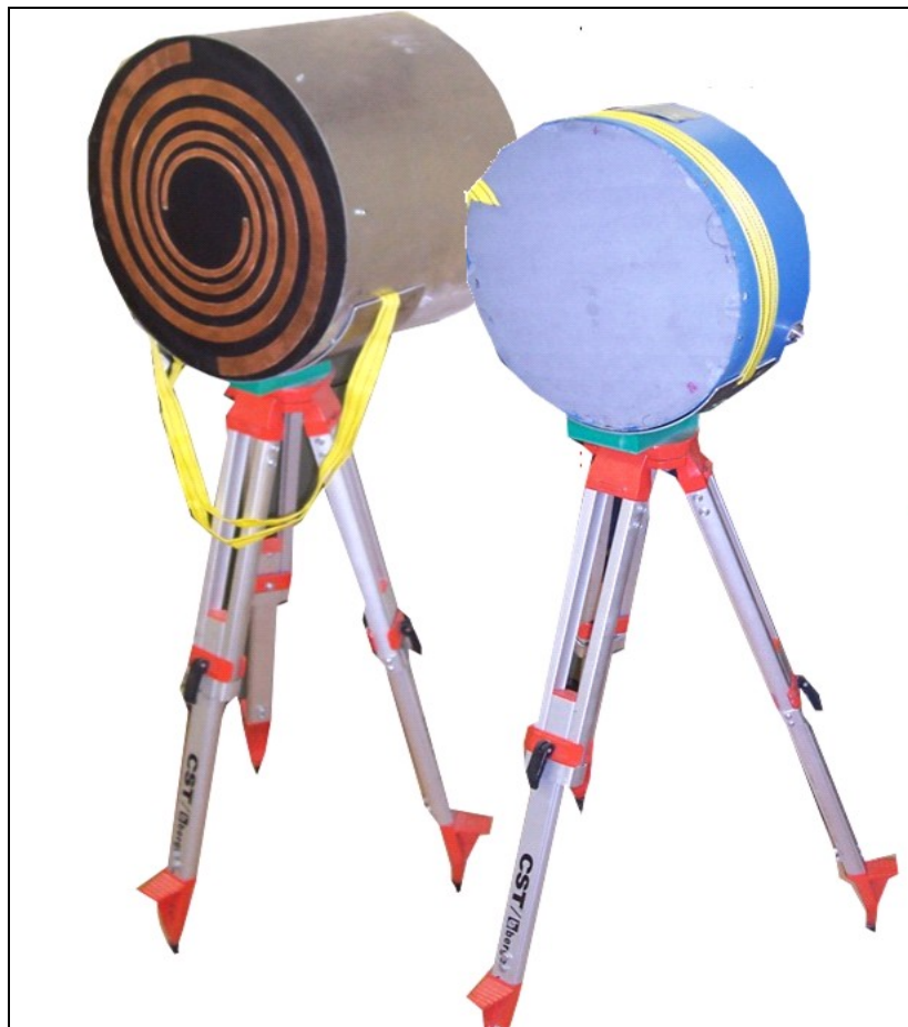
Figure 3-5. Prototype spiral LAR antennas (TX on left, RX on right).
