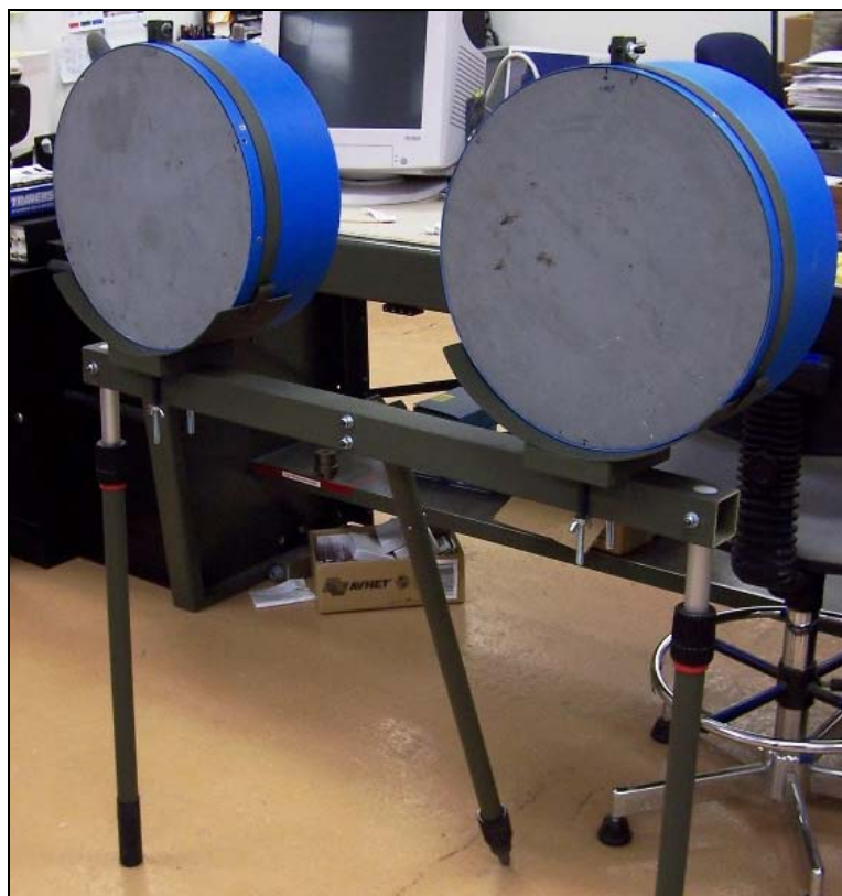
Figure 2-8. LAR radar antennas on fixed-position tripod.
