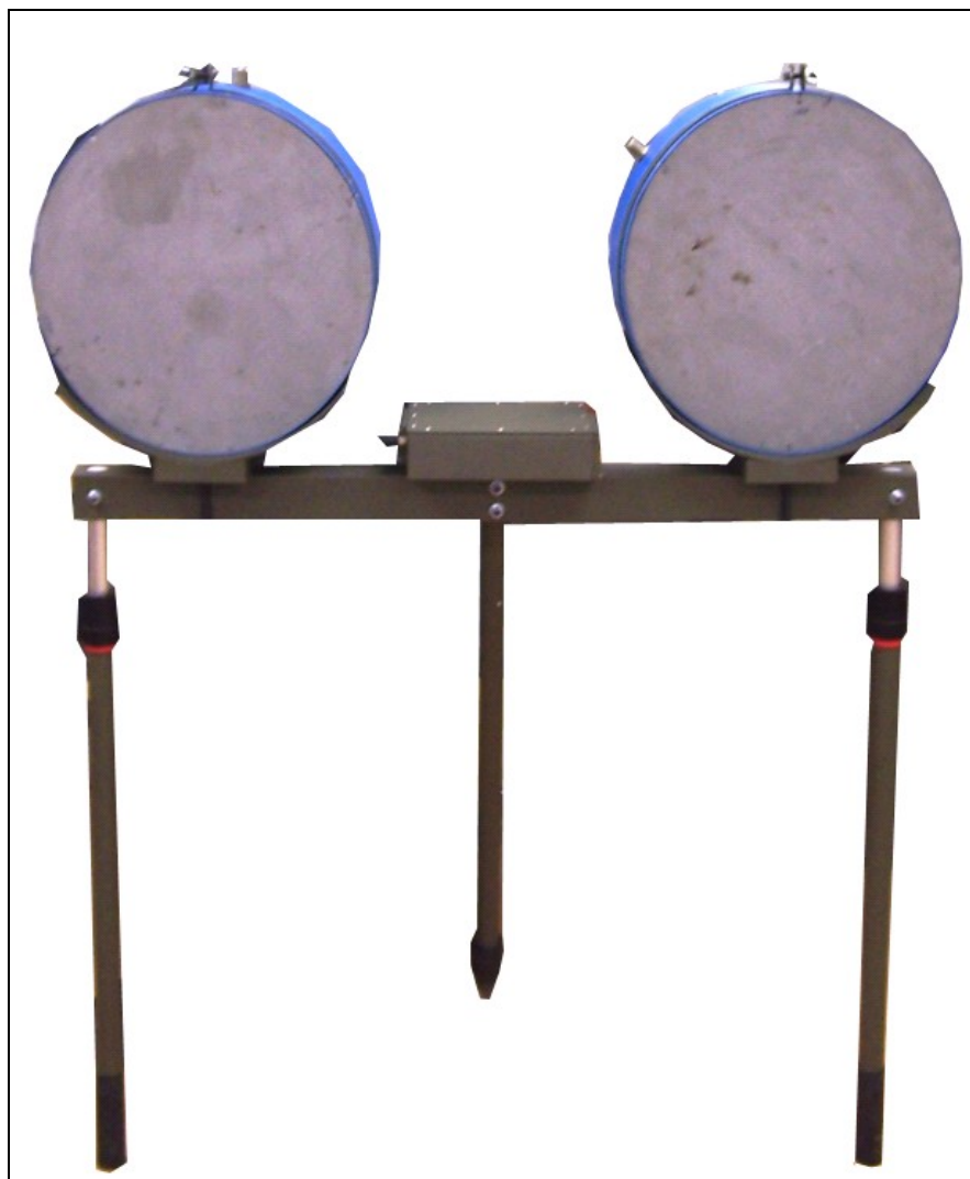
Figure 3-6. Final spiral antenna configuration for demonstration field testing.
